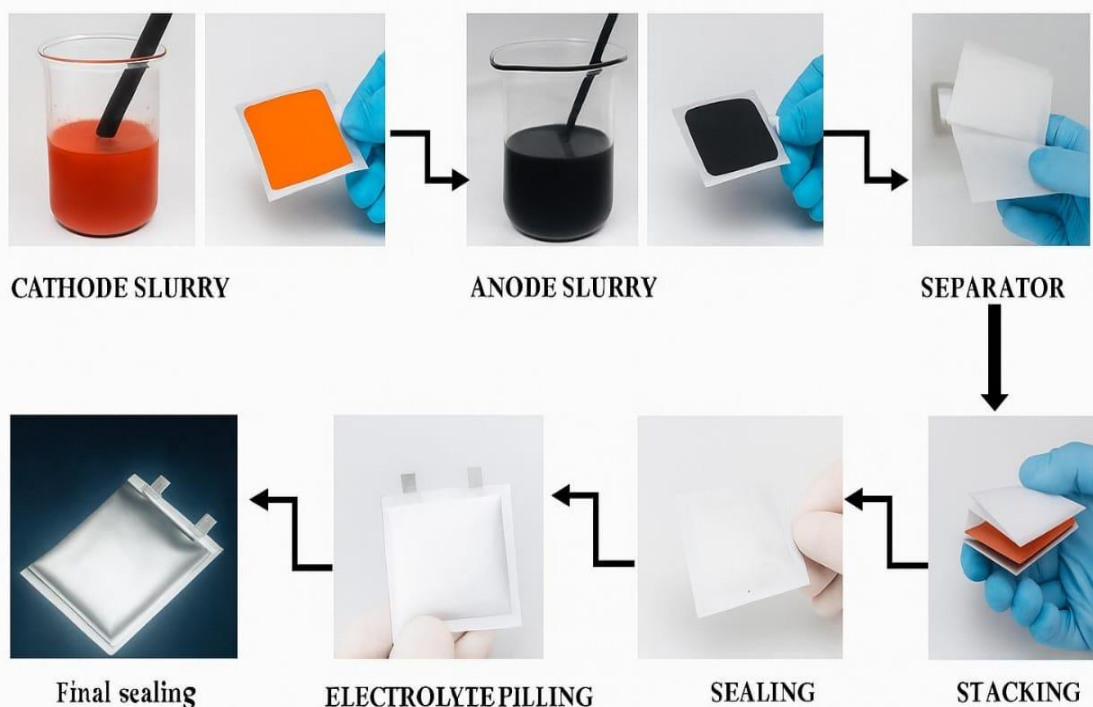
Figure1: Fabrication steps of a carbon-coated lithium iron phosphate ( \text{LiFePO}_4 ) pouch cell. The process includes preparation of the red-brown cathode slurry and black anode slurry, followed by separator stacking, pouch sealing, electrolyte filling, and final sealing of the cell
