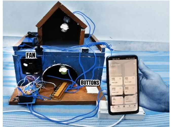
Figure 8: Shutting Down Appliances with ESP Rainmaker
