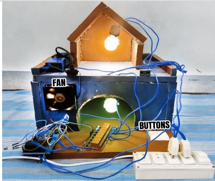
Figure 4: Turning on Appliances with Push Buttons
