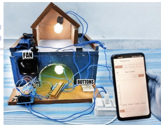
Figure 10: Monitoring Temperature with ESP Rainmaker
