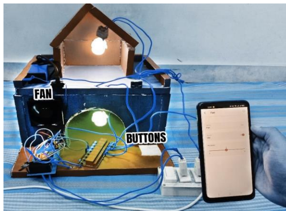
Figure 9: Controlling Fan Speed with ESP Rainmaker
