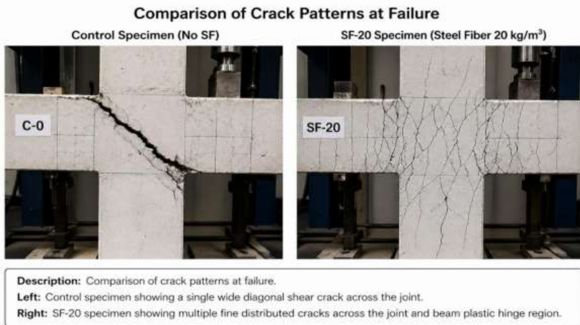
Figure 4 Comparison of crack patterns at failure.
